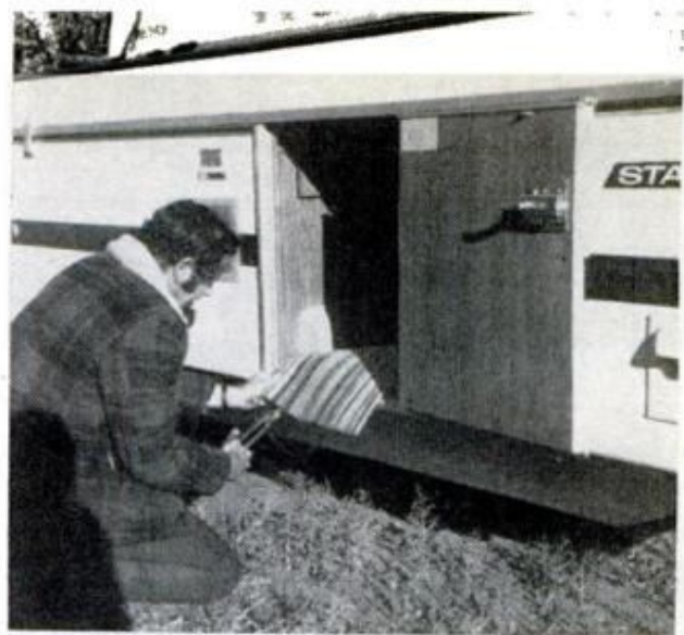
COLD FLOORS IN TENT TRAILERS can be cured with carpet remnants. Trim the carpet to fit snugly in all corners. Use two or three layers for added warmth
